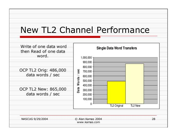
The new TL2 channel has about 75% more throughput then the original channel. This is true for burst transfers as well.
