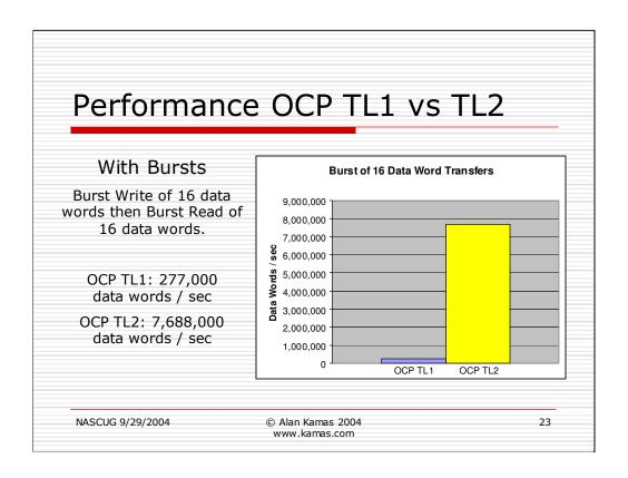
The real speed up from the TL2 channel is how it handles bursts. Here the master sends a burst 16 write command followed by a burst 16 read command, and the sequence is repeated.
