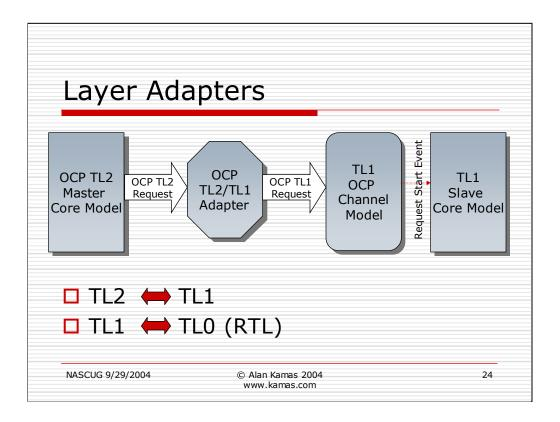
One problem with multiple channel model types is getting cores written for different models to work together.
