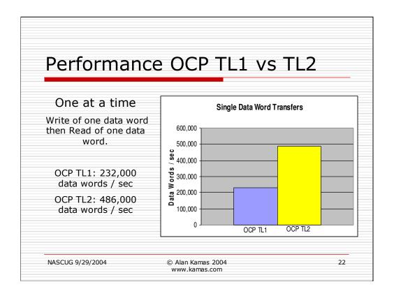
In this benchmark test the master sends a write command and then a read command. This sequence is looped 10 million times.
