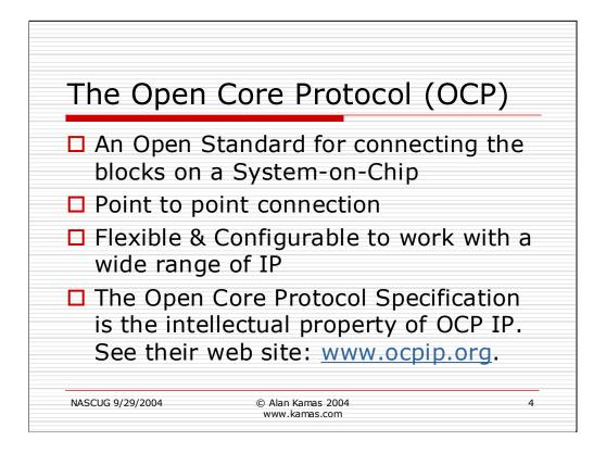
The OCP (Open Core Protocol) is an open standard for connecting the blocks of a system on chip. The Open Core Protocol is point to point – connecting one block to another – and is not a bus specification (connecting many blocks to many blocks). The standard was developed to be configurable and flexible to work with many different types of IP.
