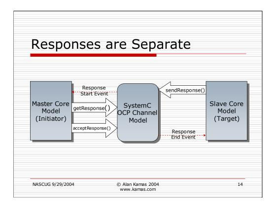
A separate path for responses allows for response pipelining.
