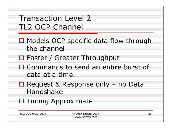
The OCP Transaction Level 2 channel is designed to work at a higher abstraction level. The phase structure is simplified, consolidating the data handshake phase into the request group. The request and response groups are expanded so that an entire burst of OCP transfers may be sent with a single command. The TL2 channel has better performance and greater throughput but the downside is that the timing will not be cycle accurate as it is in TL1.
