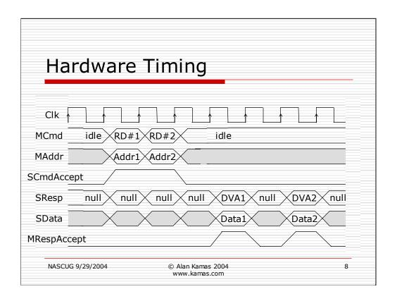
One interesting aspect of the OCP connection is that it allows responses to be pipelined. That is, it is possible to send a number of requests before receiving any responses. Here, read request #1 is sent, and then read request #2 is sent and then the response #1 is sent and then response #2. The responses may be sent anytime after the request has been received. Conceivably, this could be a long time after. The only restriction is that responses are returned in the same order as the requests.
