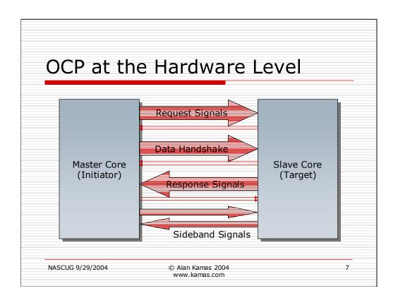
So, what does this OCP connection look like? At the hardware level, the Open Core Protocol is a collection of signals between the two cores. There is a handshake path for requests, another (optional) handshake path for request data, and a separate path for responses (which includes the response data). Note that there are also a set of sideband signals between the cores. These signals include interrupt, flags, and error signaling.
