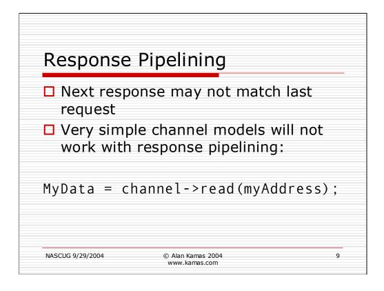
Jumping ahead here, one aspect of pipelined responses is that it limits the type of SystemC model you can have. Blocking calls like this one: myData = read( myAddress );
